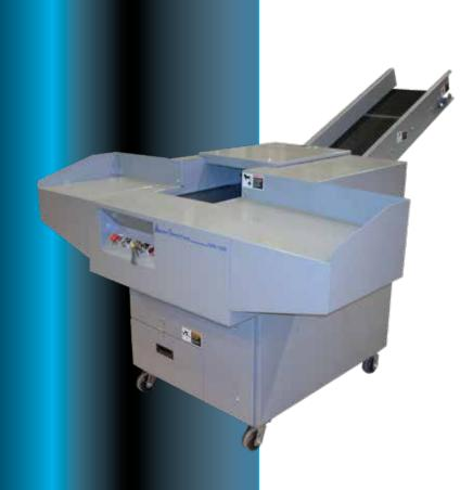
Infeed Width In Inches Shred Width in Inches 1/8" x 5/8" Throughput (Lbs per hour) 300-500 1660 Weight (lbs) Speed (FPM) 59/36/47.5 Size L/W/H in Inches Precision Ground A-2 Steel Cutters, Bag Holder, Standard Features Extra Large Feed Table, Heavy Duty Casters Available Options Auto Lubrication, Output Conveyor, Cart Tipper \* Single & Three Phase Power - Single Phase
