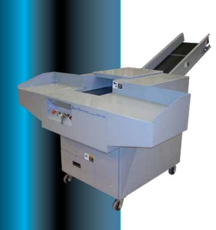
. In Voltage Motor Output In HP 3 Infeed Width In Inches Shred Width in Inches 1/4" x 1 7/8" 350-600 Throughput (Lbs per hour) Weight (lbs) 1600 Speed (FPM) 59/36/47.5 Size L/W/H in Inches Standard Features Precision Ground A-2 Steel Cutters, Bag Holder, Extra Large Feed Table, Heavy Duty Casters Auto Lubrication, Output Conveyor, Cart Tipper Available Options Notes \* Single & Three Phase Power - Single Phase Power Reduces Throughput.
