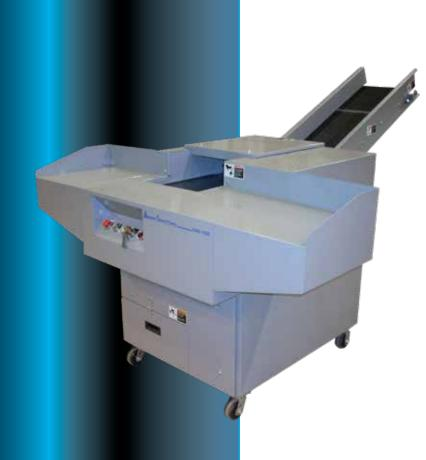
Motor Output In HP Infeed Width In Inches 1/8" x 5/8" Shred Width in Inches Throughput (Lbs per hour) 250-450 1600 Weight (lbs) Speed (FPM) Size L/W/H in Inches 59/36/47.5 Precision Ground A-2 Steel Cutters, Bag Holder, Standard Features Extra Large Feed Table, Heavy Duty Casters Available Options Auto Lubrication, Output Conveyor, Cart Tipper \* Single & Three Phase Power - Single Phase
