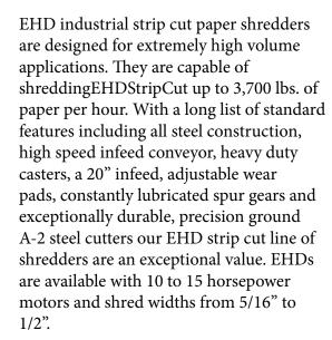
**SPECIFICATIONS** EHD1000/10B Power Requirements 208,230,460\* In Voltage Motor Output In HP 16" Infeed Width In Inches Shred Width in Inches 3/8" Throughput (Lbs per hour) 2,000-2,300 3000 Weight (lbs) Speed (FPM) 76/84/56\*\* Size L/W/H in Inches Adjustable Wear Pads, Spur Gears Run In An oil Standard Features Bath, Heavy Duty Casters Auto Lubrication, Ouput Conveyor, Cart Tipper **Available Options** \* Three Phase Power Only Notes \*\* Width Dimension Includes Side Feed Tables
